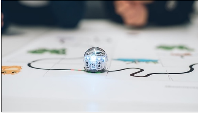
Fig. 2. An Ozobot robot following a black line.
