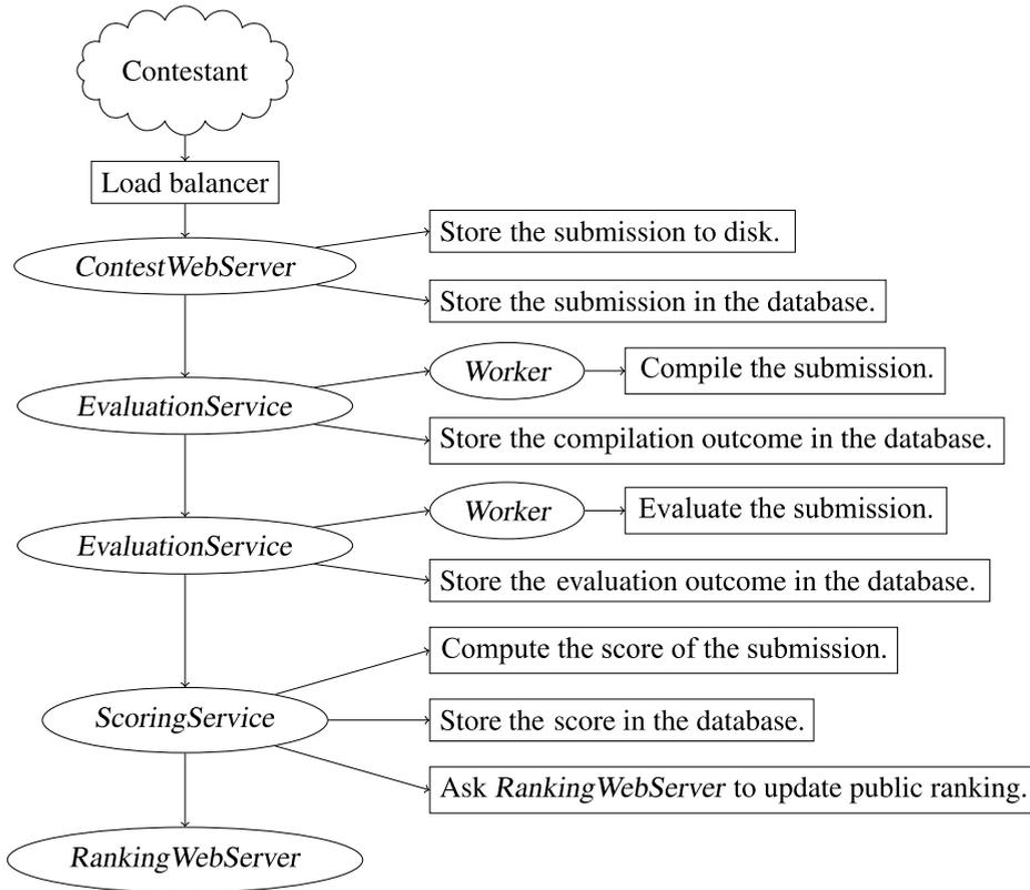
Fig. 2. Data flow of a submission through CMS.
