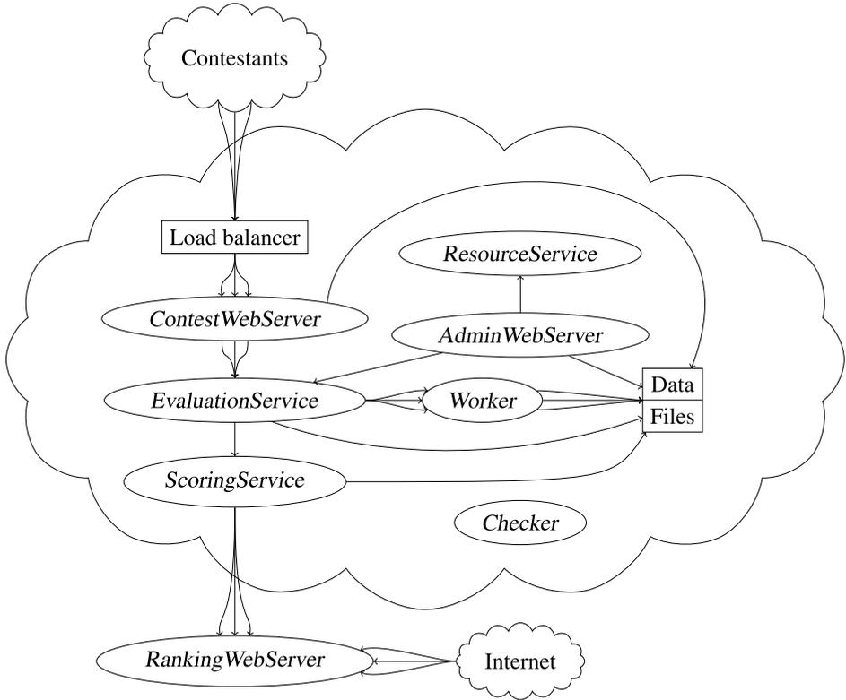
Fig. 1. Services and their interactions in CMS. An arrows represent a request of some kind, and multiple arrow heads mean that the service can be replicated. The services *Checker* and *ResourceService* talks with all the other services, and the relative arrows are omitted.
