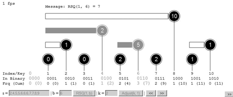
Fig. 3. Binary indexed (Fenwick) tree visualization.
