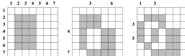
Fig. 3. Screen after each of three successive XOR operations.
